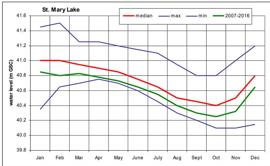
Figure 3.7 Monthly water level variations for measurements from 1978-2006. The green line shows the median water level after the weir was constructed in 2006 (2007-2015).
