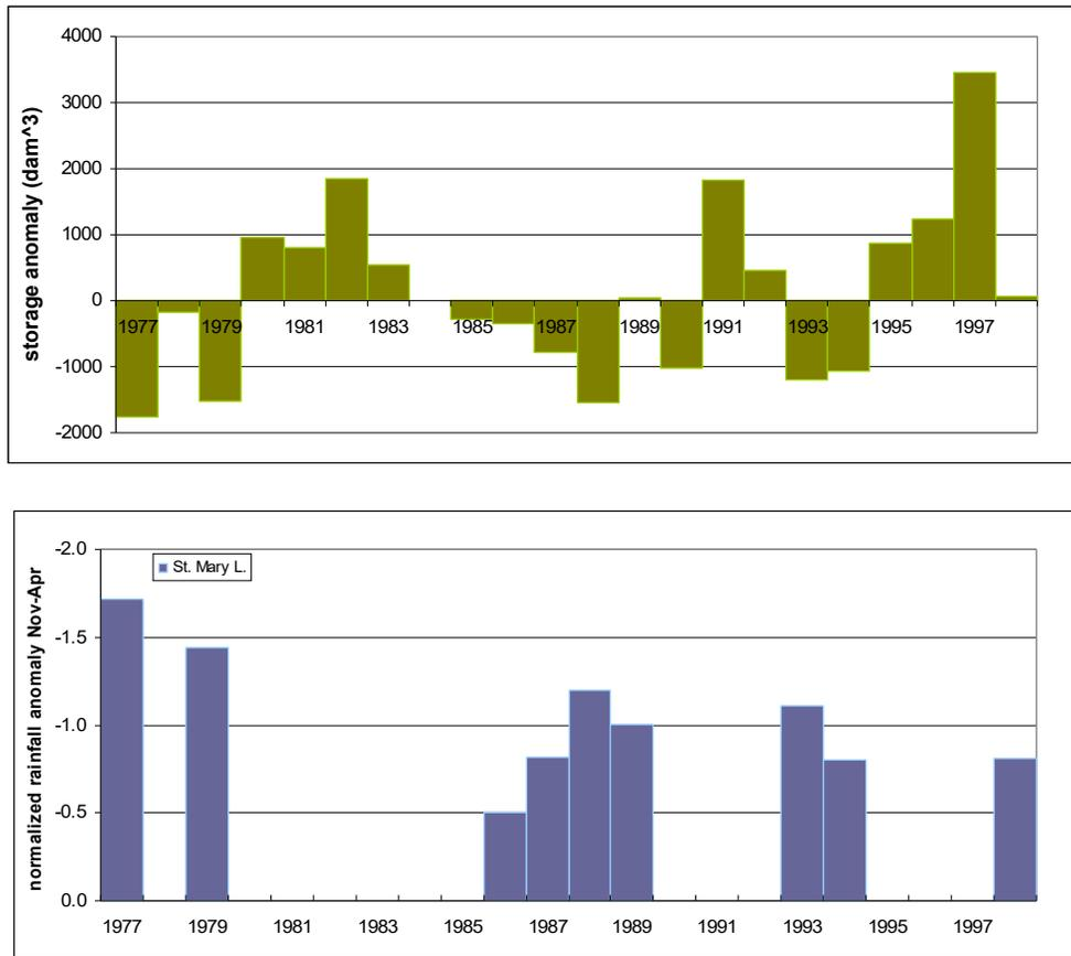
Figure 3.3 November-April discharge anomalies calculated annually for Cusheon Lake (upper panel), and corresponding precipitation anomalies for extreme low rainfall winters (lower panel).
