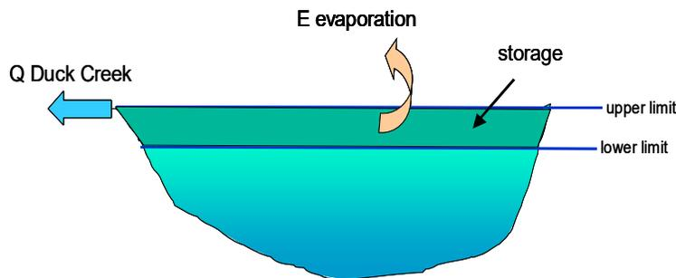
Figure 2.1 Schematic diagram for a lake reservoir showing storage between upper and lower limits. In this case St. Mary Lake flows out into Duck Creek, a fish-bearing stream.
