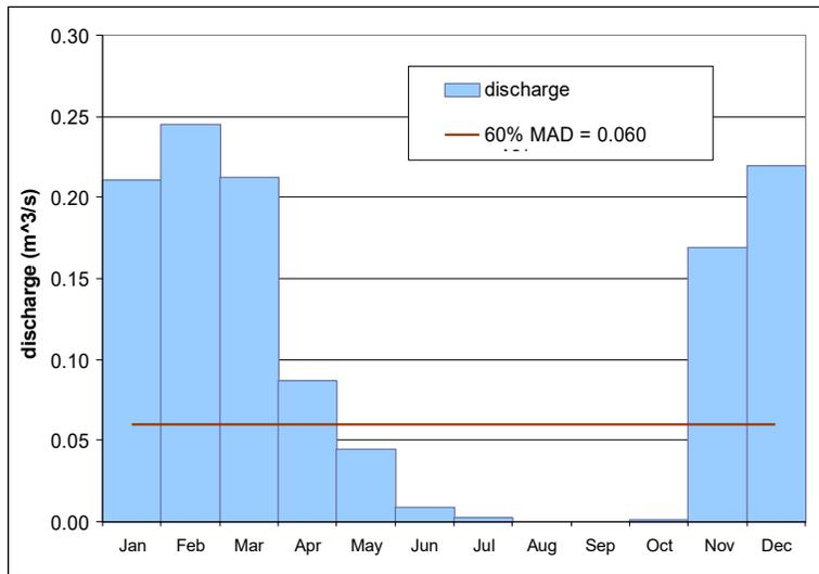
Figure 3.6 Monthly mean flows in Duck Creek derived from all measurements. The November and December data were derived by scaling January flows using ratios derived from Cusheon Lake.
